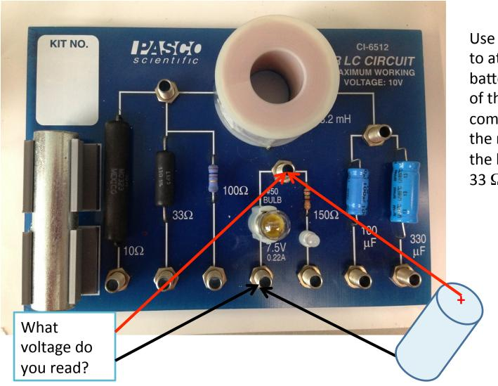
Use patch cords to attach the battery to some of the other combinations of the resistors on the left (10  $\Omega$ , 33  $\Omega$  and 100  $\Omega$ )
