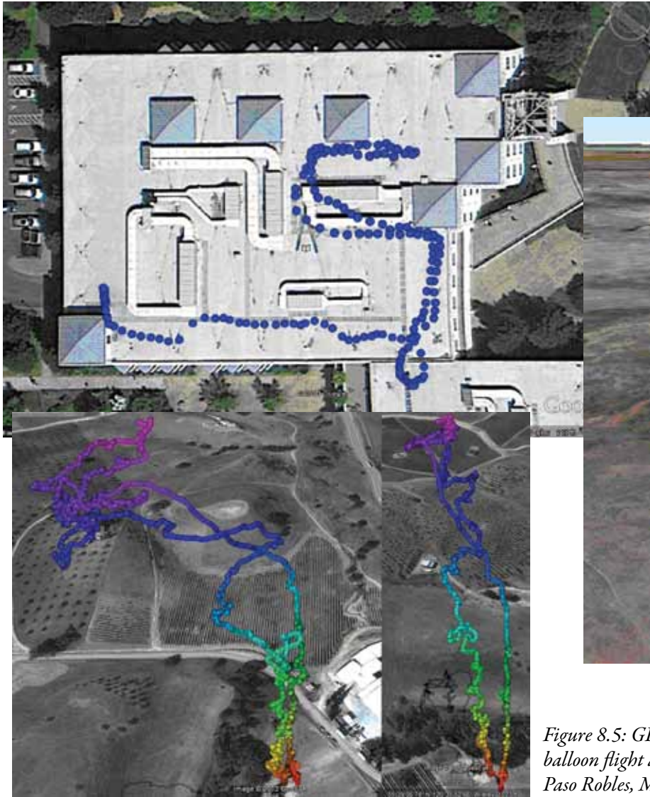
Figure 8.3: Actual path from GPS positions of the payload during a test walk around the SSU Schulz Information Center (home of the S4 team)
