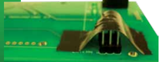
Figure 5.15: How to tape header pins to ensure even solder joints
