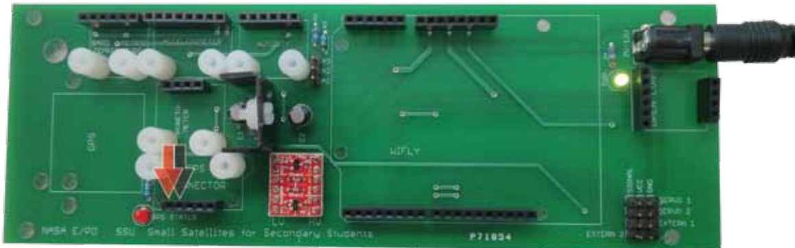
Figure 5.43: Testing the power to the GPS pins
