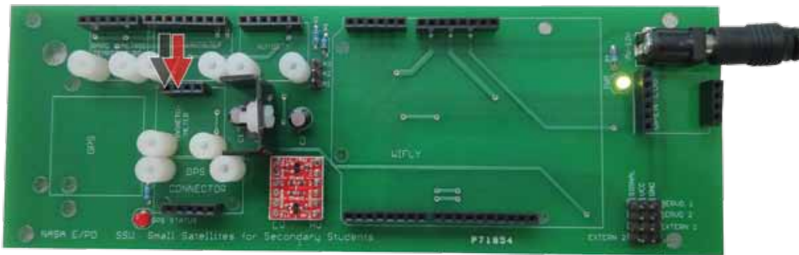
Figure 5.40: Testing the power to the magnetometer sensor pins
