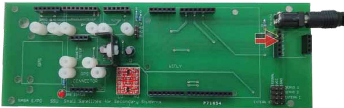
Figure 5.41: Testing the power to the Open Log pins
