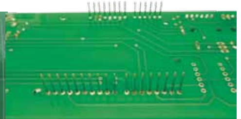
Figure 5.26: the underside of the flight board showing the uncut Arduino header pins.
